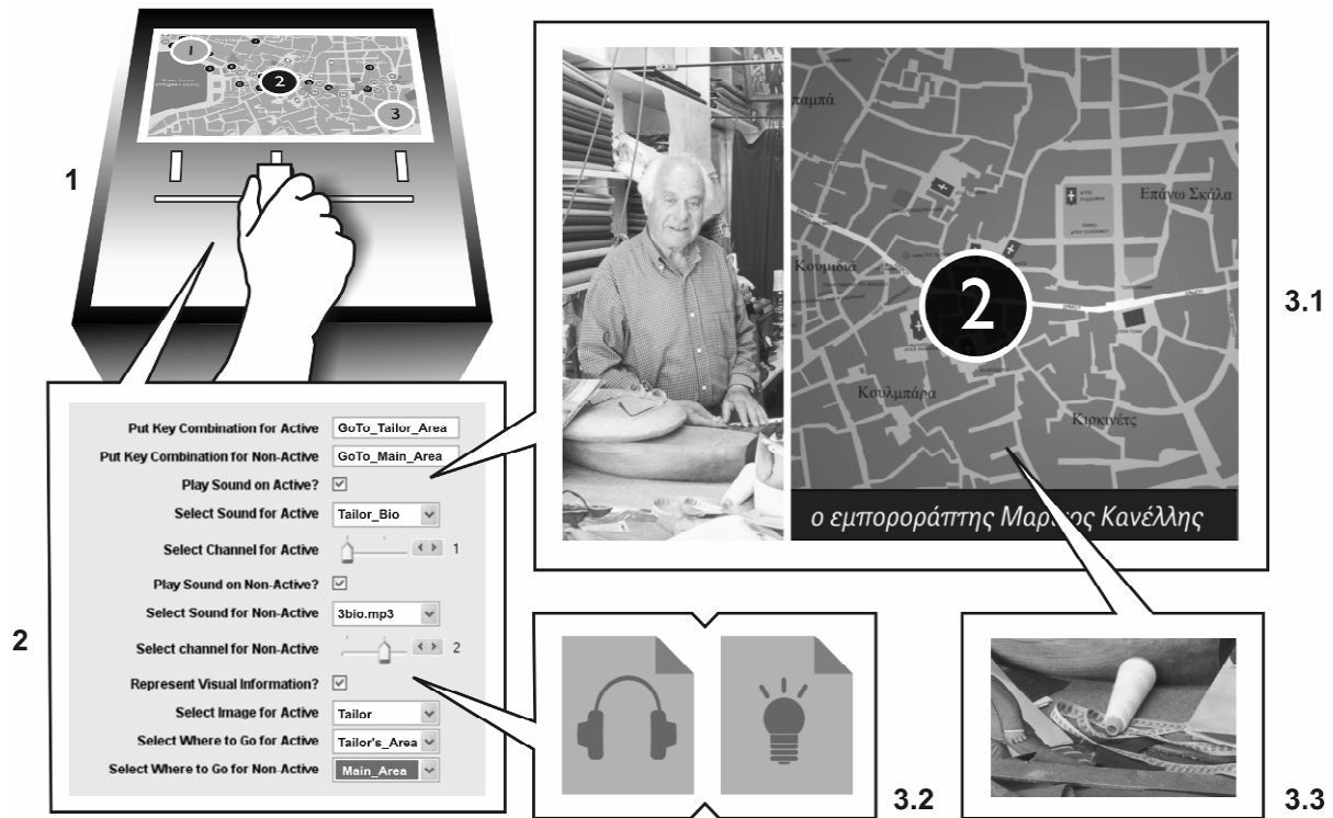
Fig. 21: The mode of interaction with the application of area E was achieved by three contact switches located at the backside of the moving cursor. According to the selection, a specially arranged area was illuminated corresponding to the figure of the practitioner at his working place with his tools and equipment of his work
